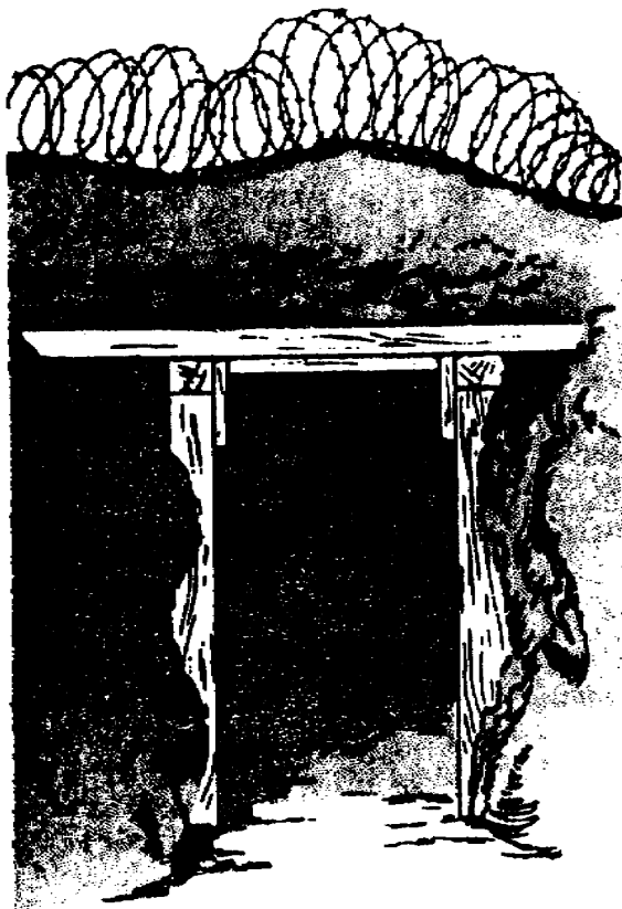
Figure 4-2. Protective wire on top of overhead cover.
